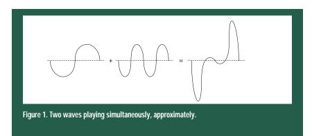
the amplitude of the wave at a specific point in time with a number from -127to 128. To mix two such waves into a third buffer, the mixer steps through each wave's 11,025 samples and adds them together, storing the result in a third 11,025-byte block to be played out through the speaker. This is the elemental mixing operation: adding two waves.
