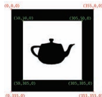
FIGURE 5 (top) To calculate a matrix that relates these two images, take the image from the camera's plane of vision and convert it to one of the pattern's four rotation poses. FIGURE 6 (bottom) shows the eight vertex values.
