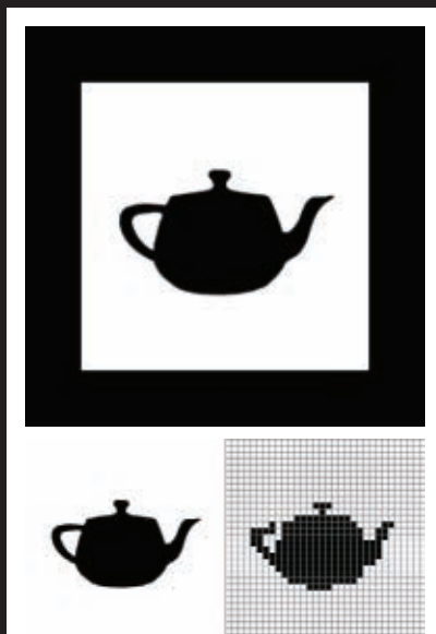
FIGURE 1 (top) shows the format for a basic pattern card. FIGURE 2 (bottom left) shows the original image and its binary representation (bottom right).
